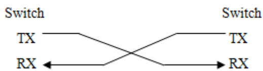
Figure 7-4 Fiber-Optic Cable Connection
